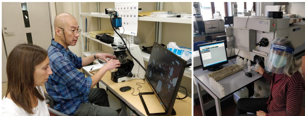
Figure 2: The analysis of pottery has been carried out both at the University of Okayama in Japan (e.g. polarized optical microscopy, on the left) and at the university of Torino in Italy (e.g. ICP-OES, Induced Couple Plasma Optical Emission Spectroscopy, on the right).
